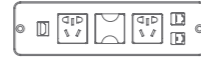
多功能插座 (选配) EFJ18 Multi-functional socket 插座模块含 2 个店员、1 个网络 (CAT.6)、 1 个电话、一个 HDMI、1 个出线模块 The socket including 2 power, Internet (Internet plug is 6 series) 1 phone, 1 VGA, and 1 flux line.
